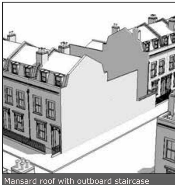
Mansard roof with outboard staircase
