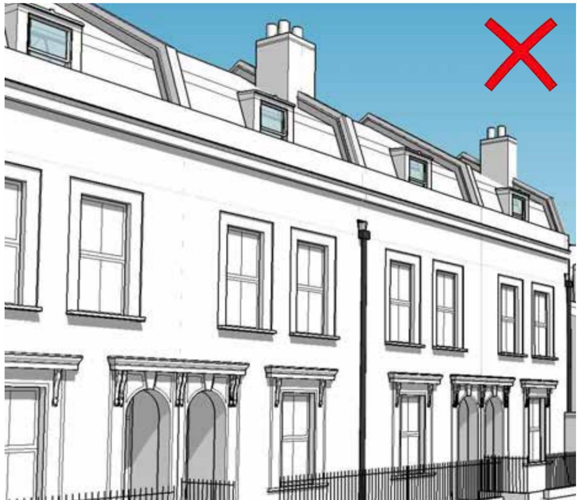
Mansard with minimum set-back to allow for gutter behind parapet wall
