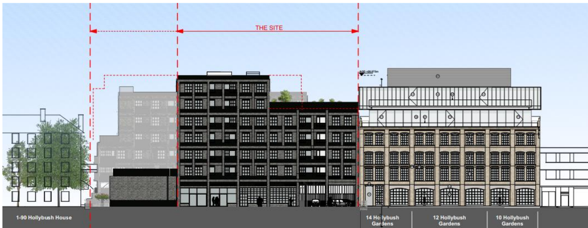
Figure 5: Proposed Block A west elevation from Hollybush Gardens with consented extension at 10-14 Hollybush Gardens shown.
