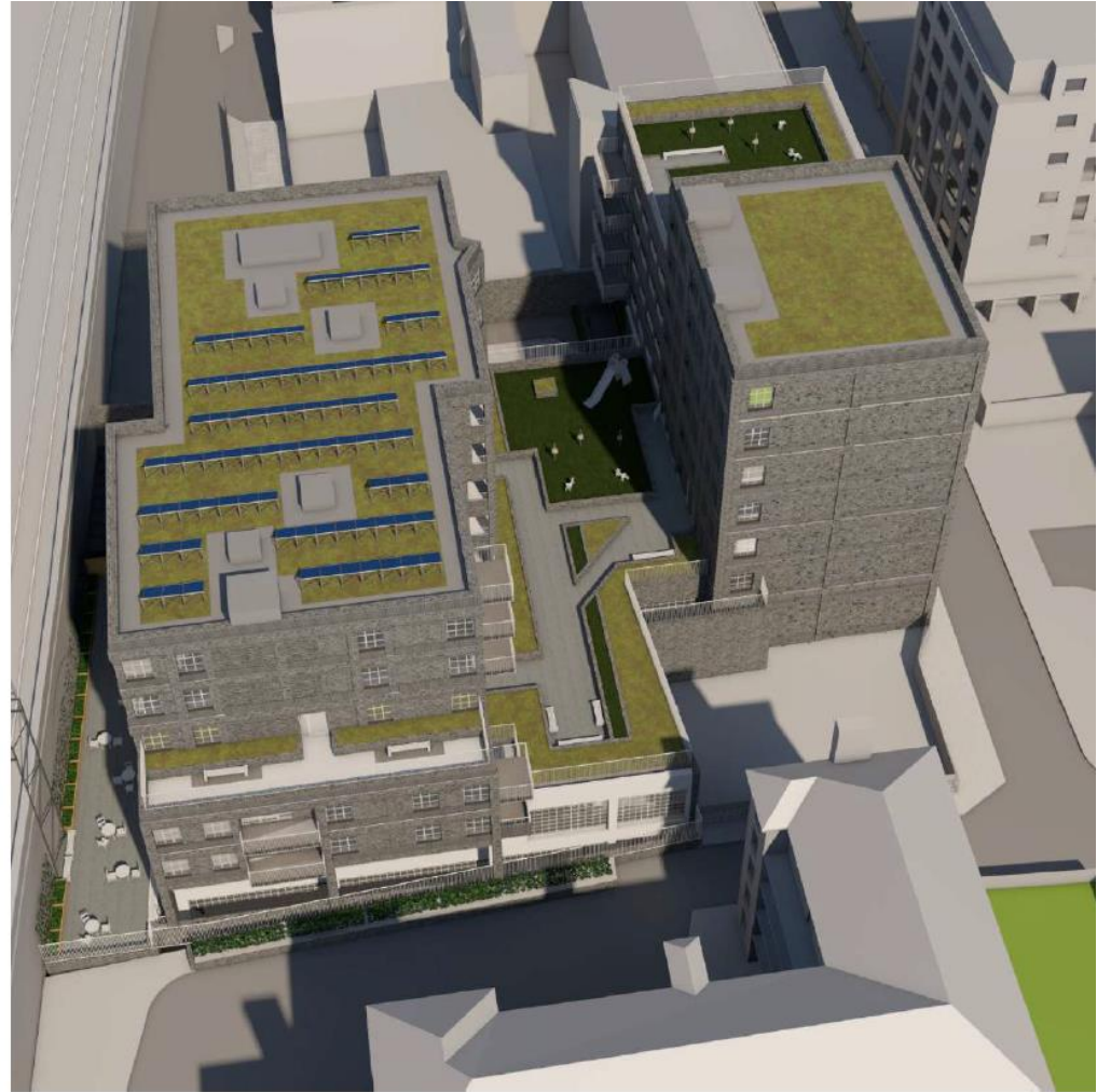
PROPOSED REVISED 3D MASSING (for clarity landscaping omitted- refer new landscape design statement)
