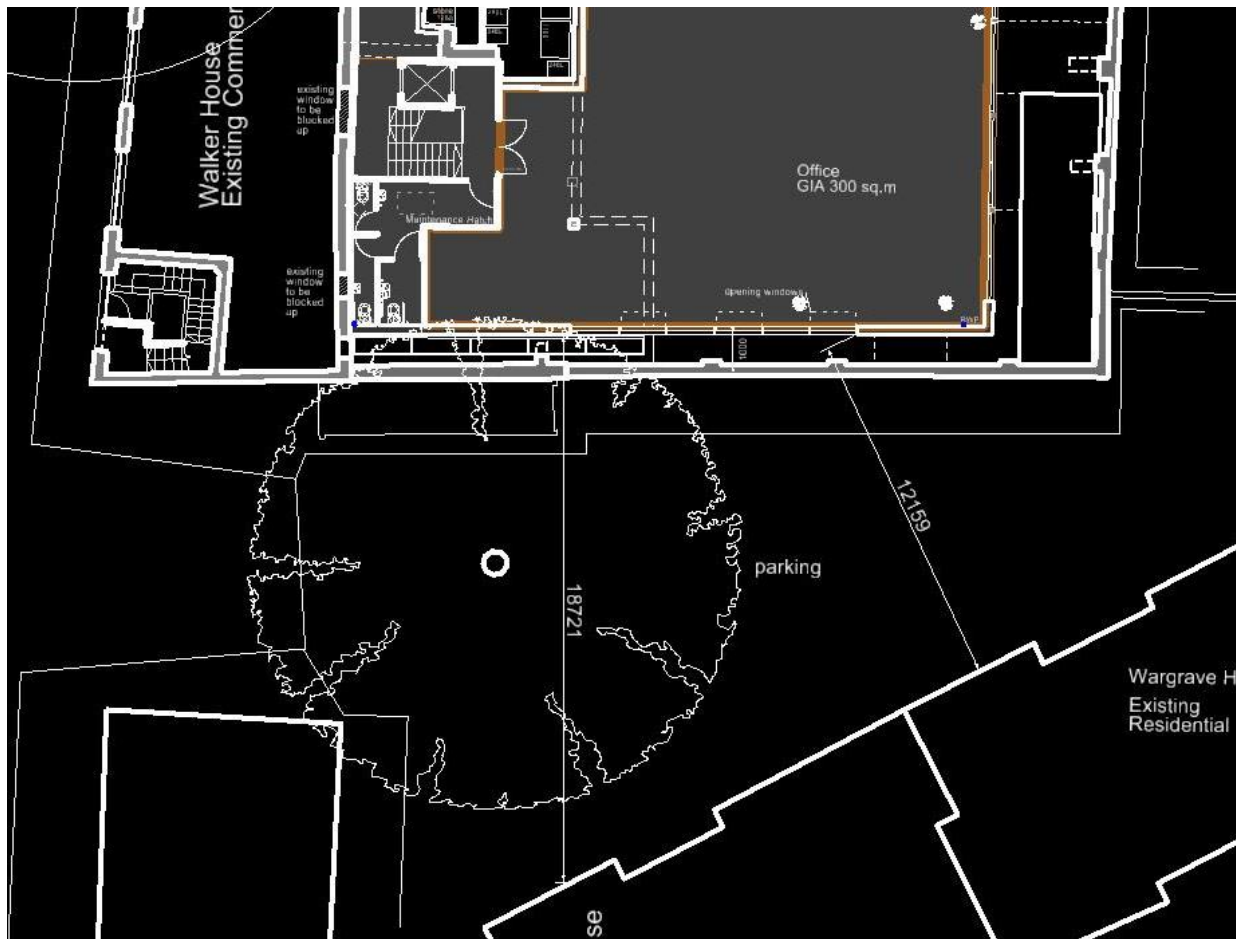
Figure 1: Diagram showing distances to Wargrave House windows. Distances are in mm.
