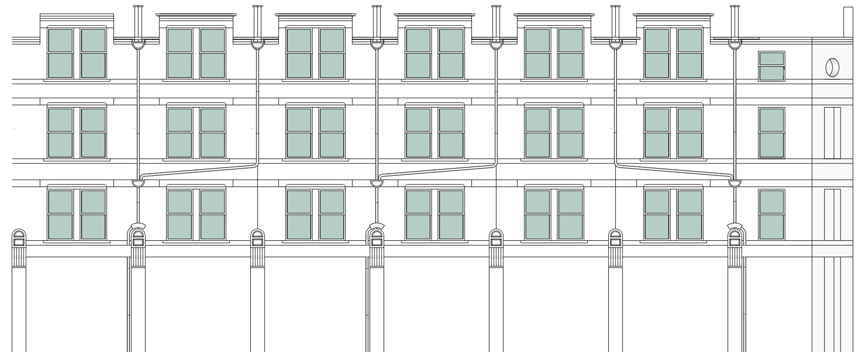
Nos.7-19 Wentworth Street Sketch of proposed facade drainage across building elevations
