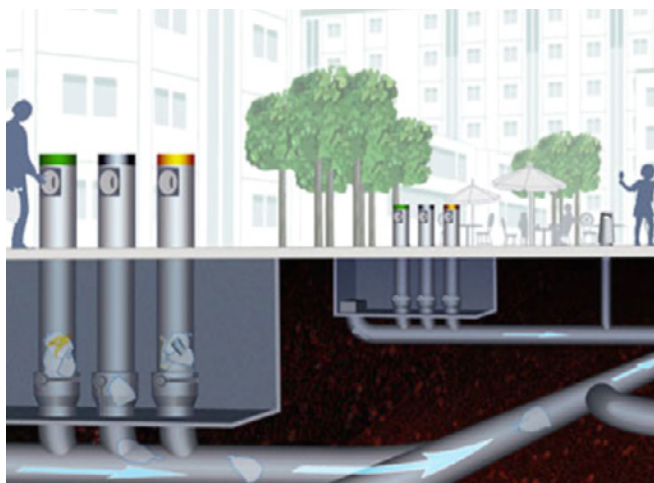
Fig. 12. Example diagram of the collection pipe system for an Automated Waste Collection System. Image courtesy of Envac.
