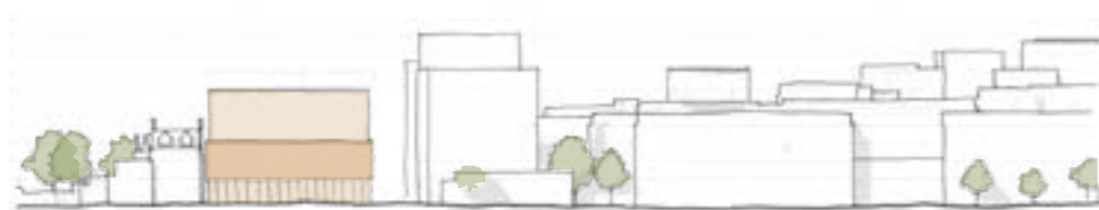
Illustrative Mile End Road Elevation suggesting how new proposals could be responding to existing datums and heritage assets
