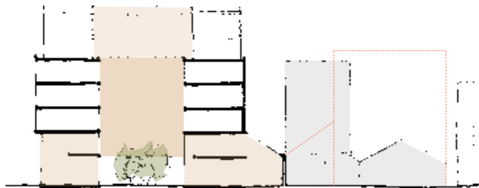
Illustrative section through the boundary wall indicating a potential approach to integrating space into the building i.e. joining the university building and hospital building to the wall to create a double height indoor space
