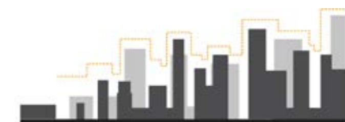
Figure 53: Create a varied and dynamic skyline with visible breaks between buildings and avoiding a terraced approach to transitioning from Tall Building Zones to lower scale context
