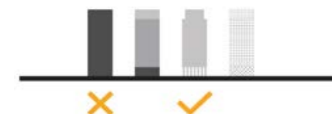
Figure 54: Create an identifiable top, middle, and bottom for tall buildings through detailing or materiality
