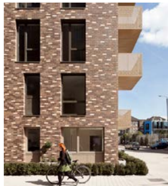
Figure 67: Ground floor entrances and windows provide activity and passive surveillance. Defensive planting area creates a semi-private zone and adds privacy. St. Andrews, London
