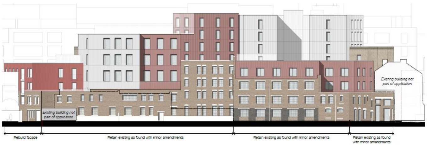
Figure 18 Proposed Pelter Street Elevation (rear elevation)
