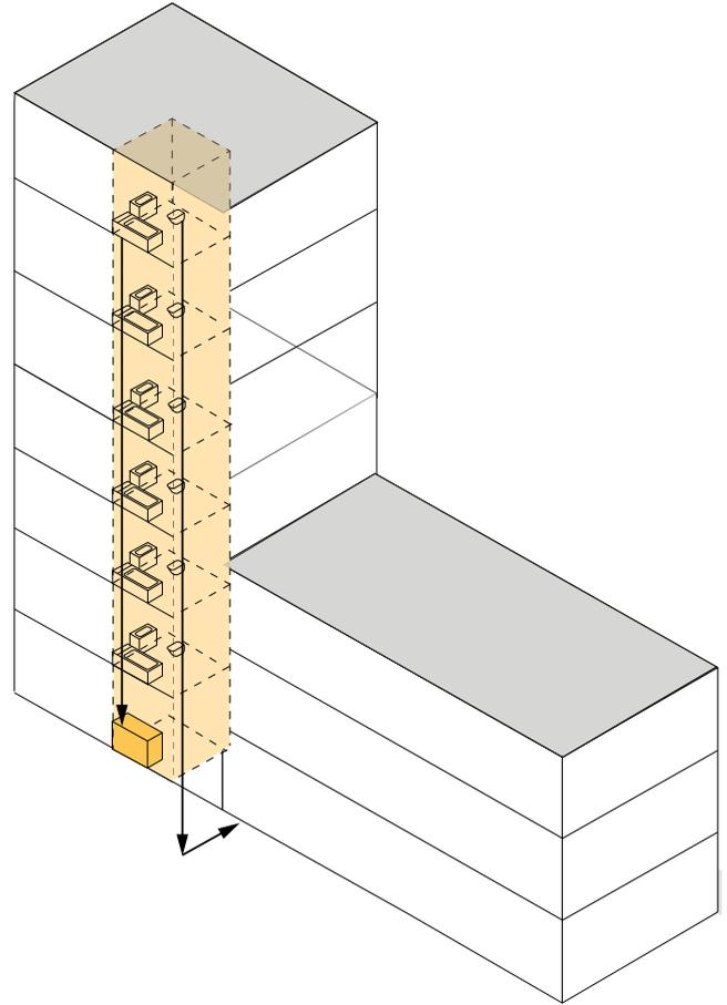
Toilets are stacked and there is sufficient space in basements/ plant rooms for the circulation of greywater.
