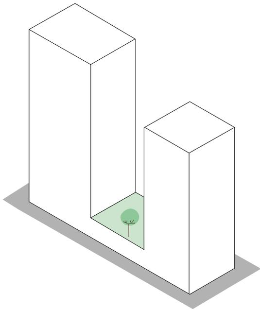
The interlinked towers typology includes a minimum of two tall forms in a single plot connected by a podium or larger mass at the lower floors. The top of the form that connects the towers typically includes outdoor communal amenity space and/ or play space.
