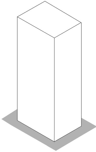
The stand-alone tower, or point block, is a single tall building that usually sits in the centre of the plot. Usually the footprint is extruded upwards but the form can also be more sculpted or include cut outs to provide additional roof tops.
