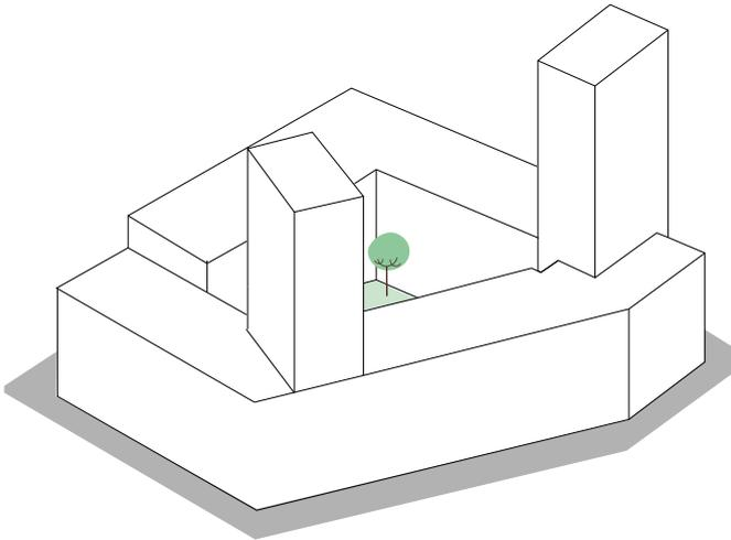
A perimeter block includes built form that wraps around the site in all directions, defining the surrounding streets with a communal courtyard in the centre. The block is not tall, less than ten stories, but can include one or more towers at different points around the
