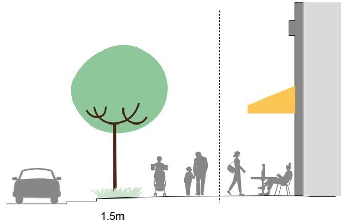
A street section. Pavements should be generous and protected from traffic with a buffer.
