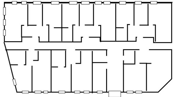
A layout of six units per core allows for a short and straight corridor with three sources of natural light. It also reduces the number of single aspect homes.
