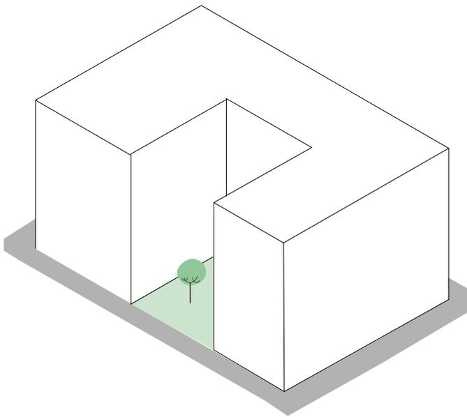
The footprint of the extruded block occupies the majority of the site and typically follows the site boundary, extruding directly upwards to form the building. Articulation or outdoor communal spaces are achieved through cutaways in the footprint, creating courtyards, or at the upper floors, creating smaller rooftop spaces.
