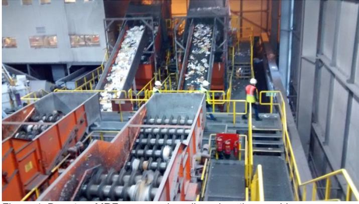
Figure 4: Bywaters MRF paper and cardboard sorting machinery
