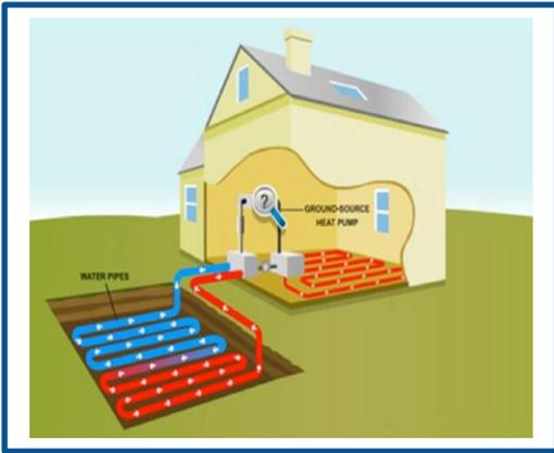
Ground source heat pump technology makes use of the energy stored in the ground surrounding (or even underneath) buildings. GSHPs are sometimes linked with geothermal energy (using either hot underground aquifers or hot dry rocks). A typical 8kW system costs £6,400-£9,600 plus the price of connection to the distribution system. There is significant potential for the use of both ground, water and air source heat pumps within the Borough
