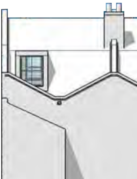
Rear parapet wall and end gable
