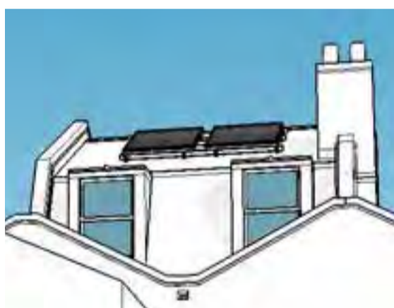
Solar panels on brackets raise the panel above the roof, making them more obtrusive in views from rear gardens
