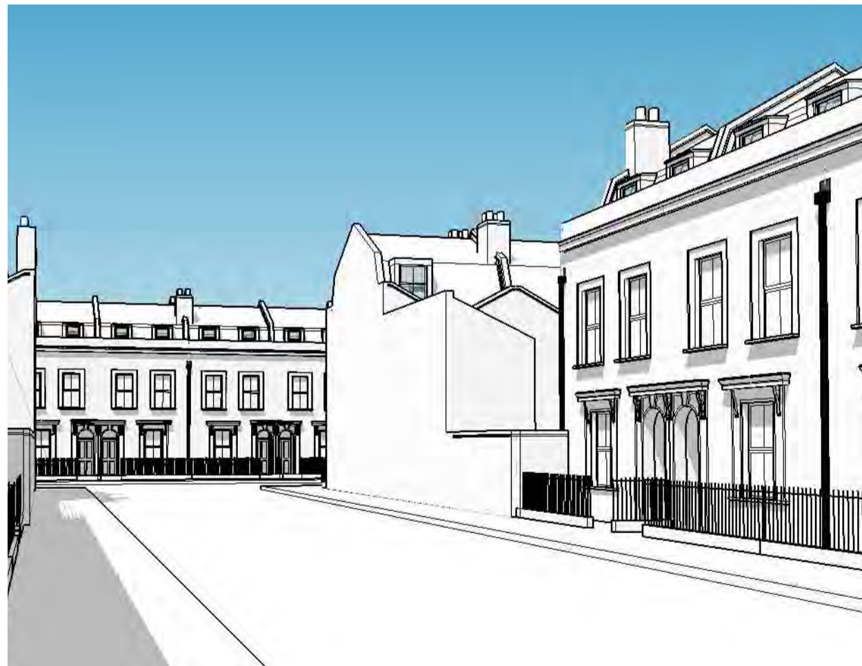
Rear view with mansard profiled gable - outboard staircase
