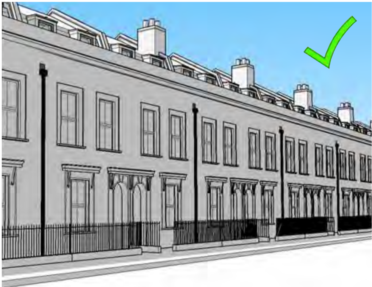
The street could maintain a unified appearance if neighbours shared a RWP
