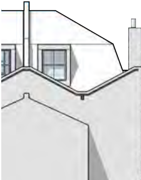
Rear parapet wall
