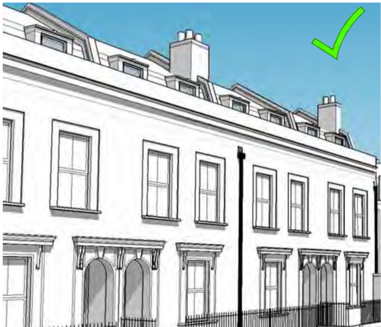
Mansard with larger set-back behind parapet wall
