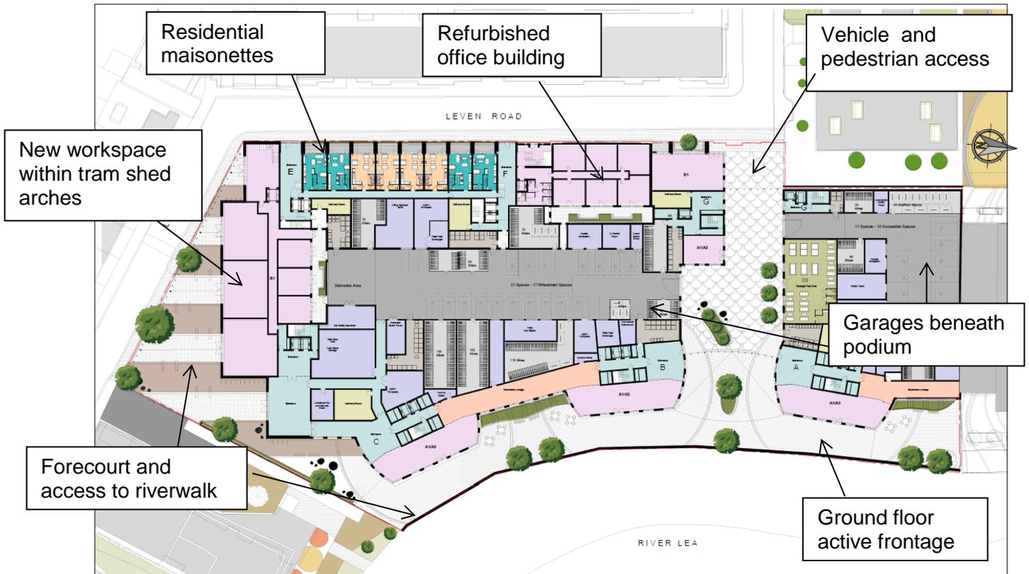
Figure 22: Annotated ground floor layout plan
